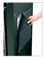
exceptionally low approach temperatures for more moisture separation at the compressor discharge and better air quality. A filter mat simplifies cooler maintenance. Dirt and dust build up on the outside of the filter, where it is easily seen and removed. This extends cooler service intervals and increases thermal reserve for harsher conditions.
